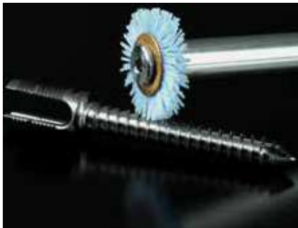
Sbavare e rifinire componenti biomedicali in titanio / Deburring and finishing of biomedical titanium components
